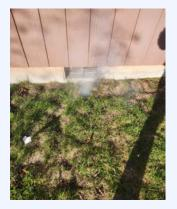
Smoke testing can also identify cross connections, where storm drains are tied into the city sewer main. By identifying and fixing cross connections, we can prevent storm water from entering the sewer system, which can overload pipes and treatment facilities. Excess storm water in the sewer system can also cause backups, overflows, added strain and on the wastewater treatment plant.
