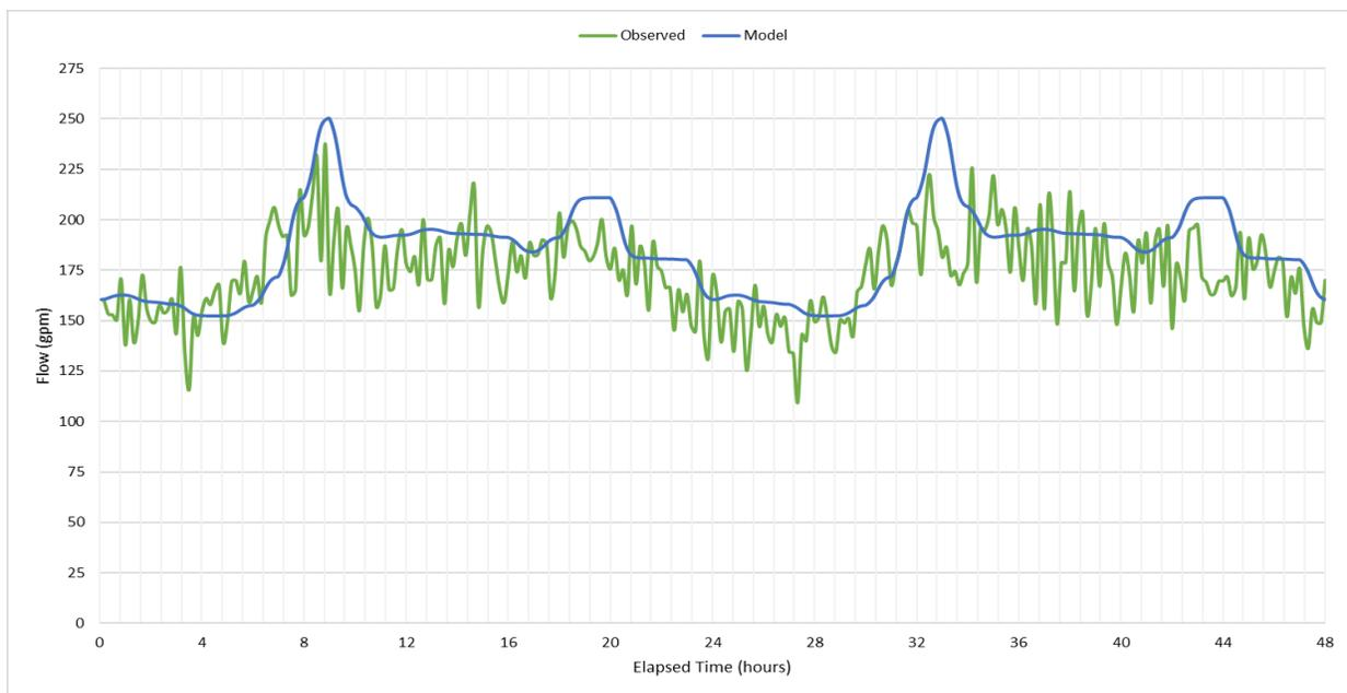
Wet Weather Flow (WWF) Calibration
