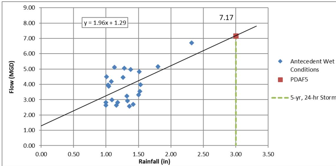
In analyzing the data, peak flows at the WWTP occurred on the same day or the following day as the storm. The PDAF<sub>5</sub> developed using DEQ’s method was compared with the top five peak day flow events from 2015-2019 (see Table 2-5 below). The PDAF<sub>5</sub> developed using DEQ’s method was selected as the value to use during this planning study because it estimates a higher PDAF<sub>5</sub> than the top five observed flow events.
